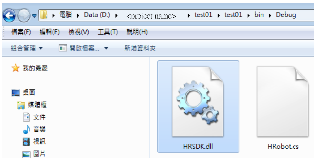
Figure 2-4 Copy the HRSDK.dll & HRobot.cs files into the specified folder
